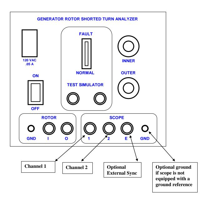
3. Power-up the instrument and the oscilloscope.
