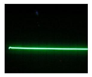
Figure 11 below shows the inverted summed single trace with the test switch closed to the fault position. In this case, the relatively large negative going blip indicates a shorted turn near the start of the simulator circuitry. If channel 1 had been inverted instead of channel 2, the fault blip would have been positive going instead of negative.
